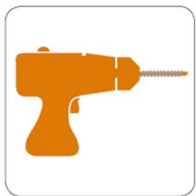
PORTABLE DRILL twist bit max 8 mm Ø
