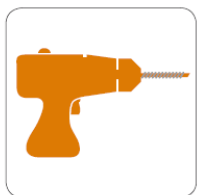
PORTABLE DRILL twist bit max 8 mm Ø
