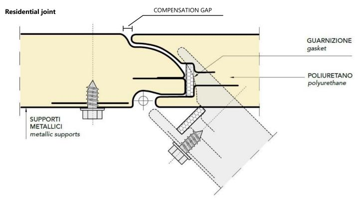
Special geometry profile which ensures that hands or other foreign bodies are not accidentally crushed during door closing, in accordance with EN 12604.
