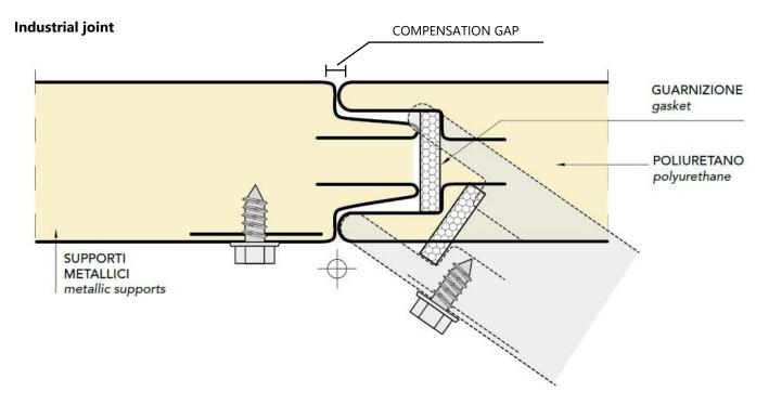
Standard joining system provided with continuous reinforcement plates, which guarantees maximum resistance to repeated opening and closing, as well as excellent resistance to the exposure of atmospheric agents.
