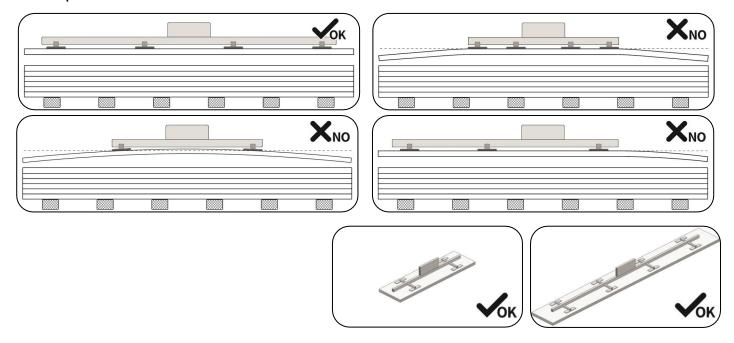
The following are, by way of example, two conceptual solutions for correct suction cup systems in which the suction cups are properly distributed according to the length of the panel.
