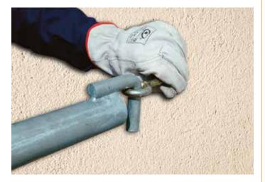
15 • inserting the anchorage
