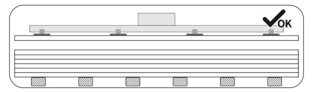
The study and analysis of the suction cup systems to be used is essential to avoid damaging the panels, so it is advisable to design suitable solutions by also discussing with the suppliers of the systems as experts in the field. Failure to design the lifting system can lead to panel breakage as a result of panel imbalance.
