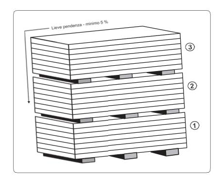
The best storage conditions are in closed, lightly ventilated, moisture-free and dust-free rooms. In any case, and in particular for storage on the construction site, it is necessary to provide a suitable, stable support surface that does not allow water to stagnate.
