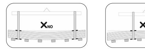
In the absence of a sling bar, in some cases unloading can also take place using suitable forklift trucks. In order to avoid damage to the panel or even breakage of the parcel, the lifting equipment must have fork spacing and fork width that take into account the parcel length, weight, and thickness of the panels that affect the bending of the parcel.
