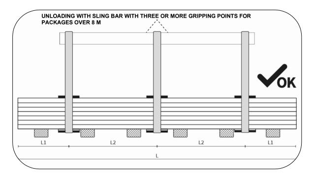
Gripping of parcels in the wrong manner such as using incorrect and/or incorrectly dimensioned gripping equipment or without considering the correct distance of the gripping points can lead to alterations and consequent damage to the panels in the parcel.
