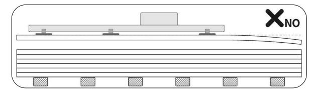
The following are, by way of example, two conceptual solutions for correct suction cup systems in which the suction cups are properly distributed according to the length of the panel.
