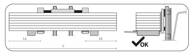
If the parcel is lifted in an unbalanced manner, not taking into account the correct gripping points, there is a risk of consequences such as the parcel falling or the panels being deformed and damaged.
